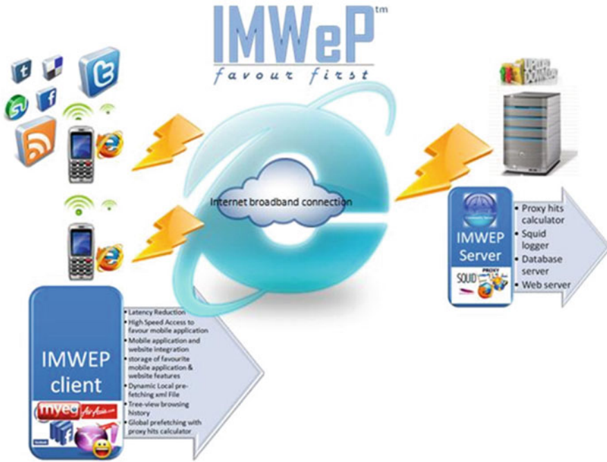
Fig. 14.1 Architecture of Web cache server and mobile clients
