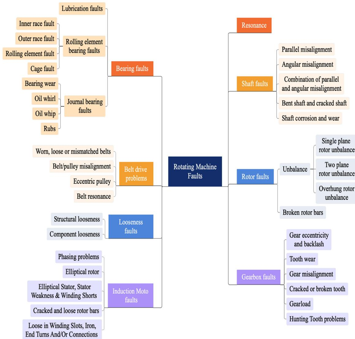
Fig. 5. General component-level faults in rotating machines.
